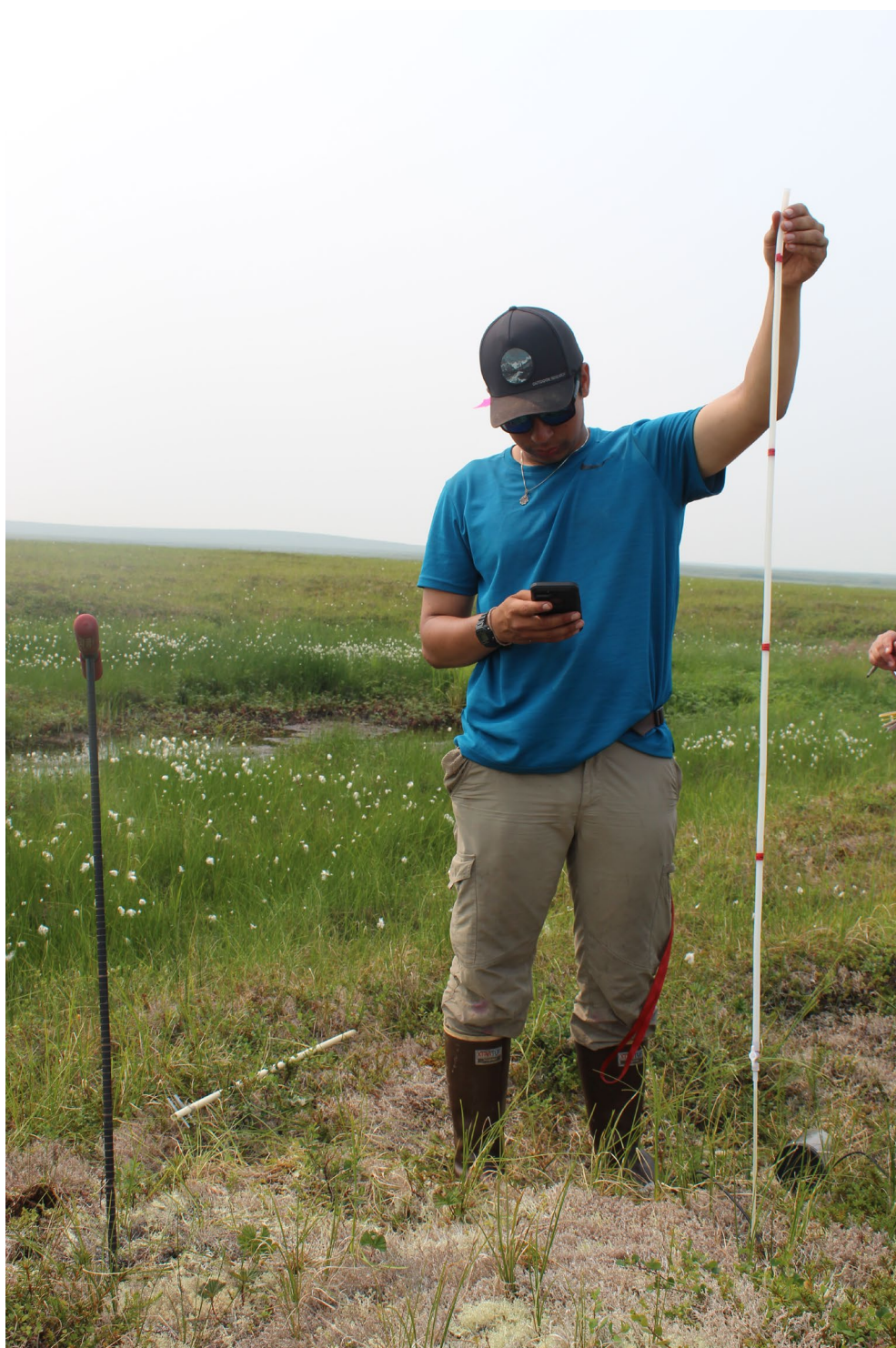
Figure 1: Sample area showing burned and unburned tundra (left); falling head hydraulic conductivity measurements (right),
