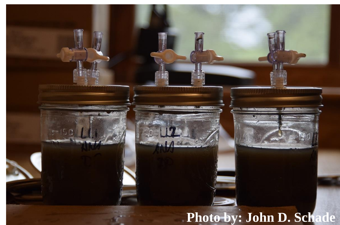
Figure 1 , Examples of aerobic incubation jars and collecting GHG flux using LGR in a channel fen site.
