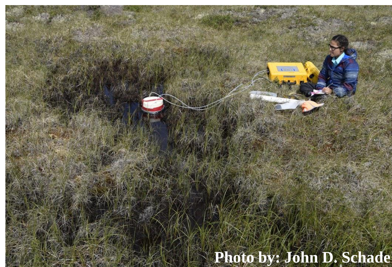
Figure 1 , Examples of aerobic incubation jars and collecting GHG flux using LGR in a channel fen site.
