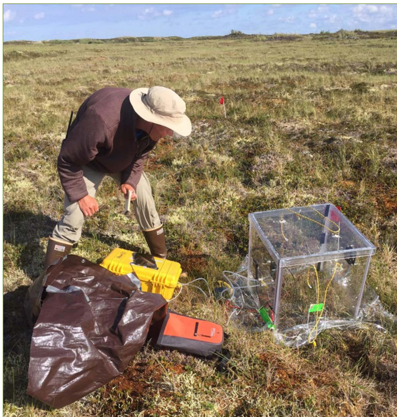
Figure 5. Licor CO 2 flux system and transparent chamber with PAR sensor, thermometer, and cover for measuring resp.
