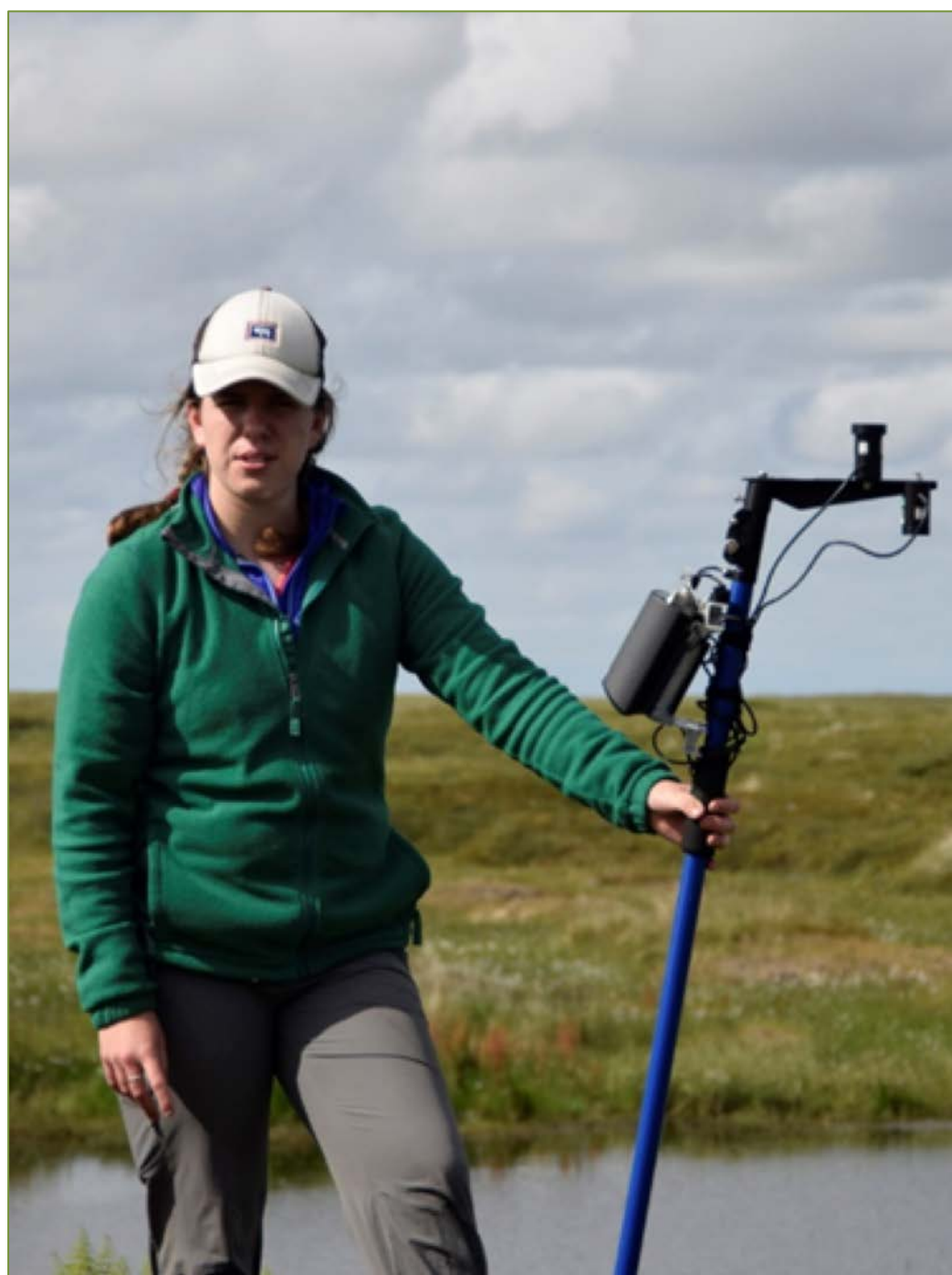
Figure 2. SKL 910/2 NDVI pole from Skye Instruments with dual sensors for measuring ground NDVI.
